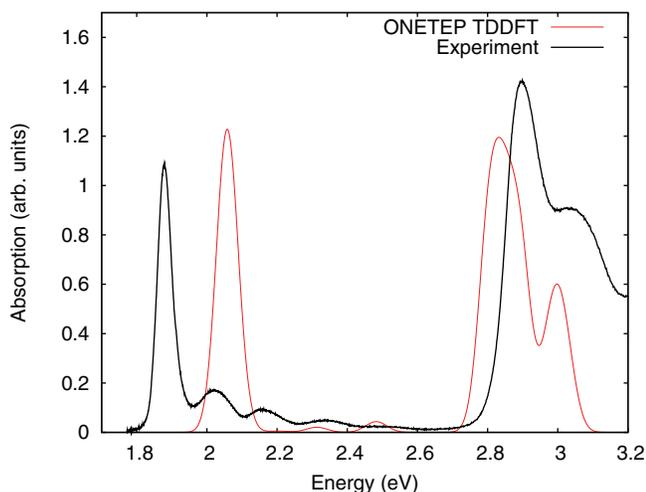
FIG. 4. Absorption spectrum of chlorophyll a generated from the 12 lowest excitation energies compared with the experimental spectrum of chlorophyll a in diethyl ether.<sup>52</sup> An artificial smearing width of 0.03 eV was used in producing the ONETEP TDDFT results.
