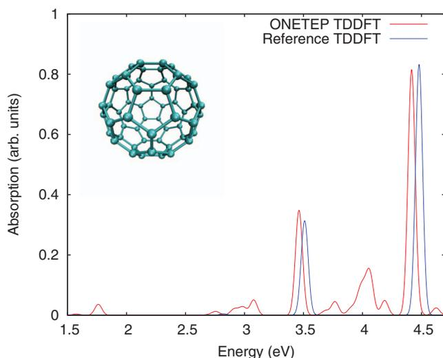
FIG. 2. Absorption spectrum of  $C_{60}$  generated from the 150 lowest excitation energies. An artificial smearing width of 0.03 eV was used in generating this plot. The positions and oscillator strengths of three major excitations were taken from Ref. 51 and are plotted here using the same artificial Gaussian smearing to produce a reference spectrum. The two spectra were scaled according to their relative oscillator strengths.
