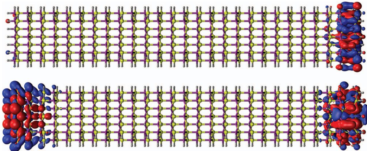
FIG. 5. The transition density of the lowest excitation of a GaAs nanorod as found for a truncated density matrix at  $75 a_0$  (upper figure) and the full density matrix (lower figure). The excited state corresponding to the truncated response density matrix is  $0.33 \text{ eV}$  higher in energy than the one corresponding to the full density matrix. In this plot, H is shown in grey, As in yellow, and Ga in purple.
